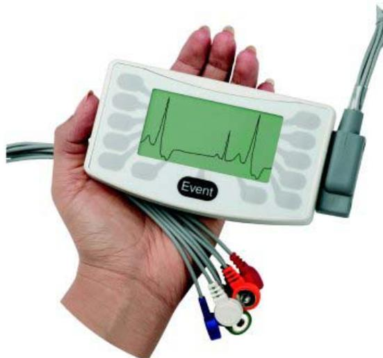
Figure 4: Holter Monitor – CardioPerfect Holter ECG
